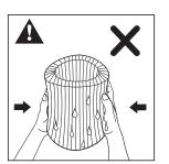
Clean the humidification filter every week. Please soak the humidification filter with mid or acid cleanser (24g citric acid with 4L water) for 1 hour.
