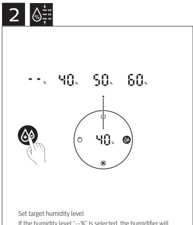
If the humidity level "--%" is selected, the humidifier will keep working until the humidity level reaches 70%RH.
