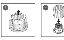
Replace the humidification filter every 6 months. The humidification filter contains a biocidal product (Active substance Zinc pyrithione CAS 13463-41-7).
