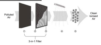
The Pre-Filter, HEPA Filter and Activated Carbon Filter are combined into one easy-to-change filter.
