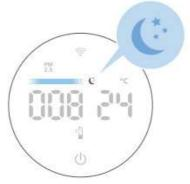
**Sleep mode ( © ):** The appliance operates quietly at a low speed. After 3 seconds, the screen's light switches off.
