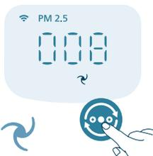
**Medium mode (↻):** In the Medium mode, the air purifier operates on a medium speed.
